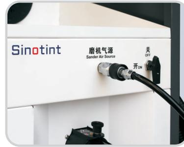
Pneumatic design, no motor, no electric wires,
